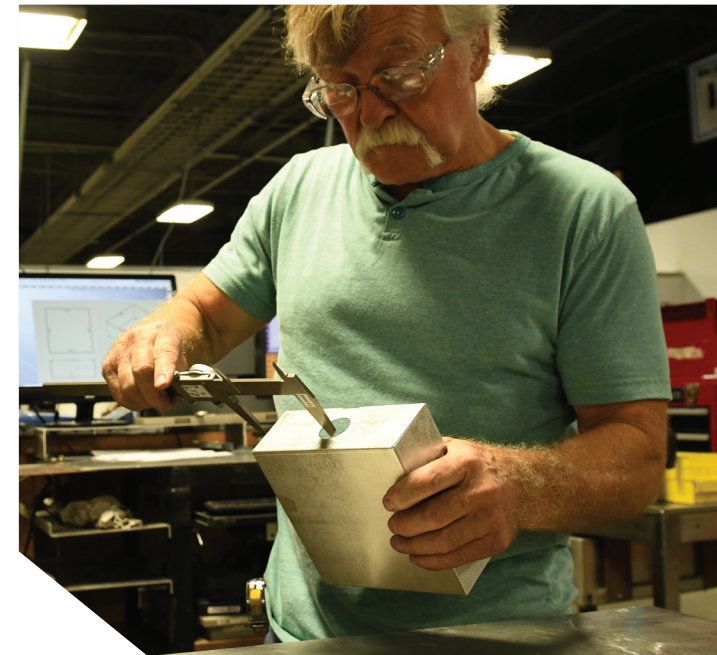
Caliper measurements for bend accuracy, are part of the entire sheet metal quality control process.
