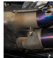
Final Material The team printed the final part in titanium for installation on the race bike to reduce weight while maintaining durability (see bottom left).
