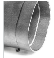
Prototype Material HDFR iterated in Stainless Steel 316L , a lower-cost material for testing the design on an engine dynamometer to ensure the new design did not impact performance.
