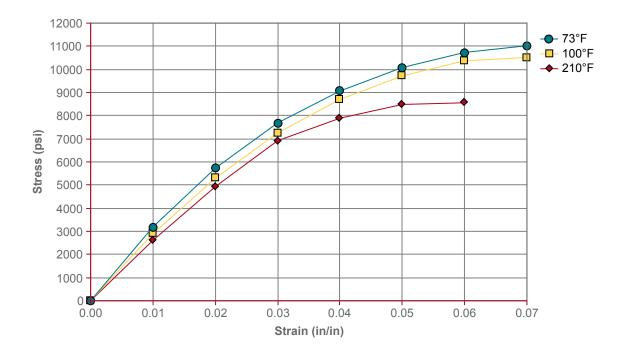
Secant Modulus vs. Strain (ISO 11403-1)
